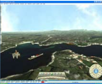
High resolution texture map draped on a DTM with 3D solid objects
