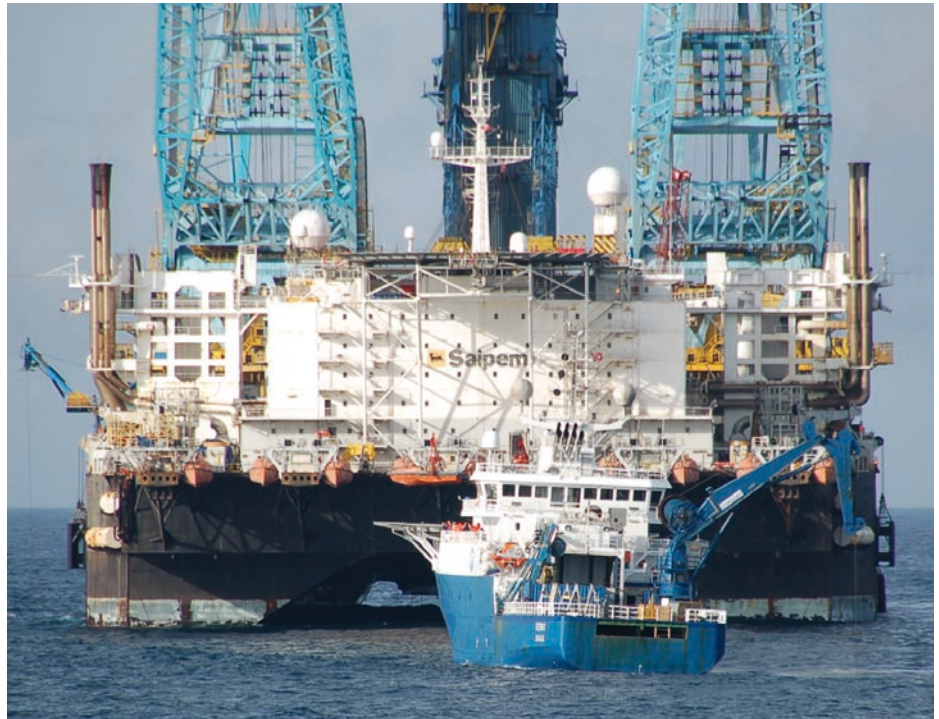
Figure 2: Geobay is a small boat. A typical offshore survey and construction scenario: SV Geobay in front of the Saipem 7000 crane and laybarge (Photo courtesy of Bo Krogh).
